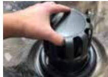
Pull Up to Remove Floater Assembly
