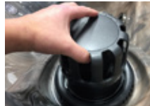
Pull Up to Remove Floater Assembly
