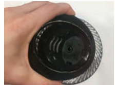
Hold Handle Firmly and Pull Up
