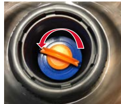
Turn Filters Counter-clockwise to Remove
