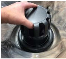
Pull Up to Remove Floater Assembly
