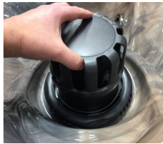
Pull Up to Remove Floater Assembly
